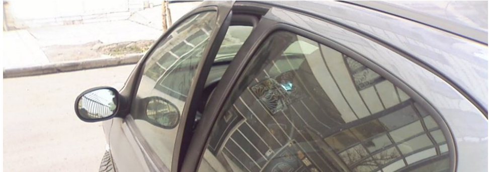
An Iranian made Peugeot 206 can be easily stolen by bending a door.
