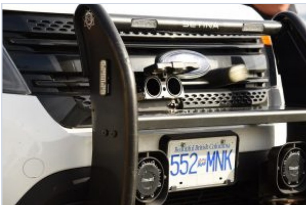
A compressed-air launcher mounted on the front of a police vehicle is ready to fire the GPS tracking projectile. (Delta Police)
