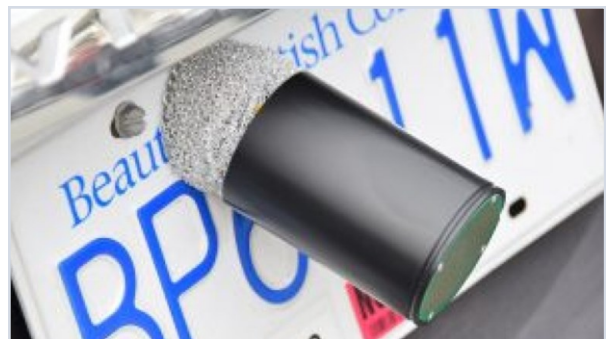
Eight Delta police vehicles are equipped with technology that can launch a GPS projectile from the grill of a police car at a suspect vehicle. The department says it will allow officers to track vehicles while not engaging in a pursuit. (Delta police)
