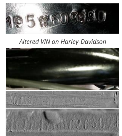
Optical, magnetic and eddy - current images of the true VIN location
